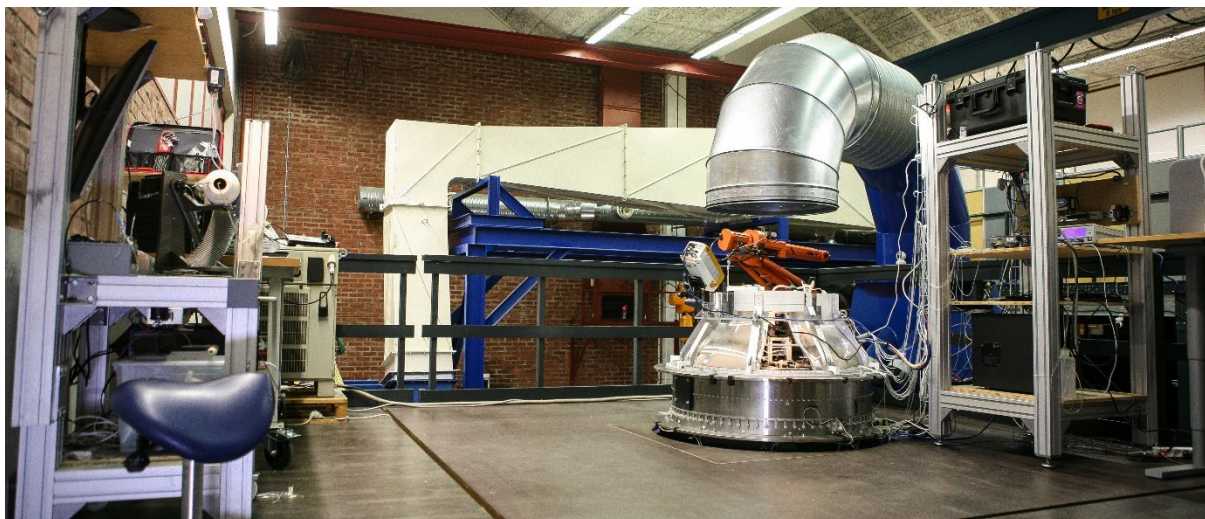
Figure 3-1 The upper floor of the new compressor facility after the completion of the experimental test campaign. The probe calibrator can be seen to the left and the IR camera mounted at the ICD outlet.
